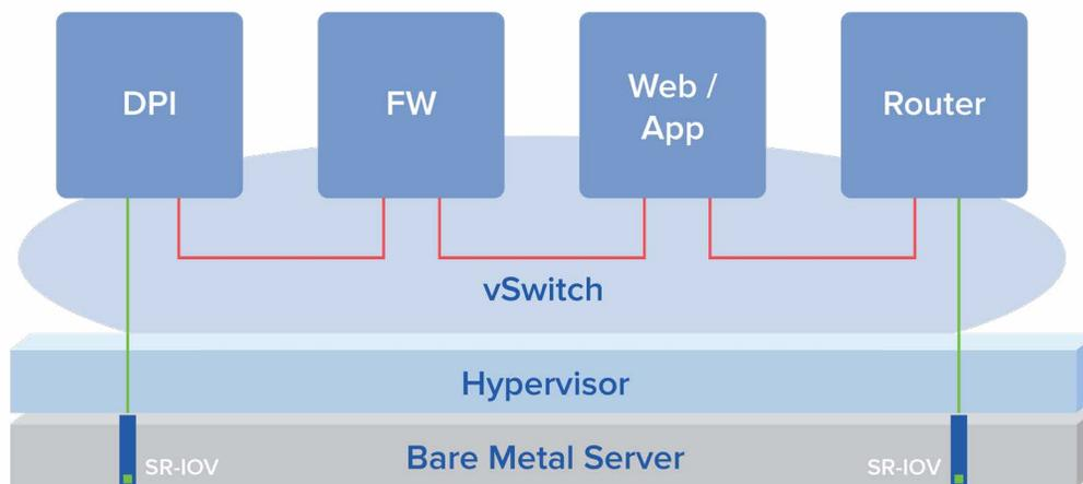
Figure 4: NFV service chain throughput bottleneck between SR-IOV and vSwitch connectivity.
