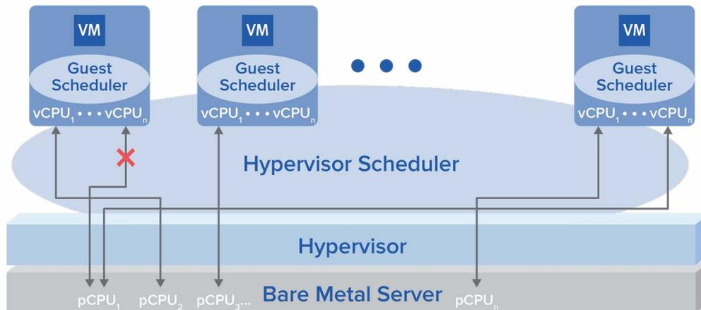
Figure 1: Blocking between two VMs on a monolithic type 1 host configured with 1-n vCPUs.
