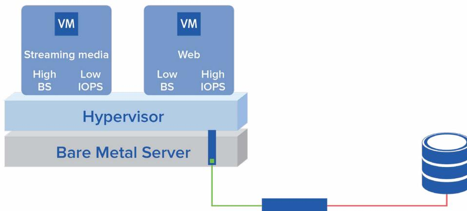
Figure 3: Impact of varying IOPS and BS profiles on volume Storage hitting same SAN target.
